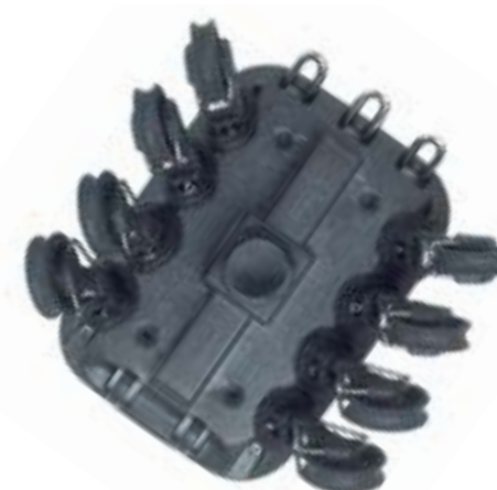
Plugged T-base. Cables exit through mast heel for deck connections.
