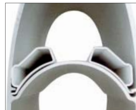
One-piece (closed) cable conduits prevent moisture from getting into cabin on keel-stepped masts.
