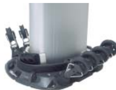
Step the mast and replace the wedge.
