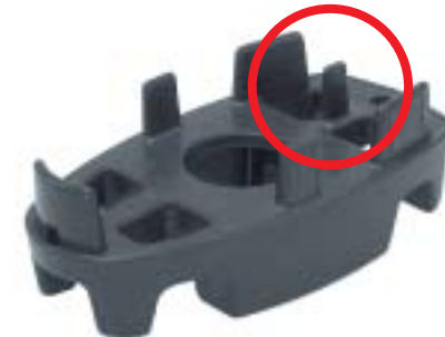
Small protrusion on top side of heel plug – acts as spacer for cable conduit. Allows cables to run freely.
