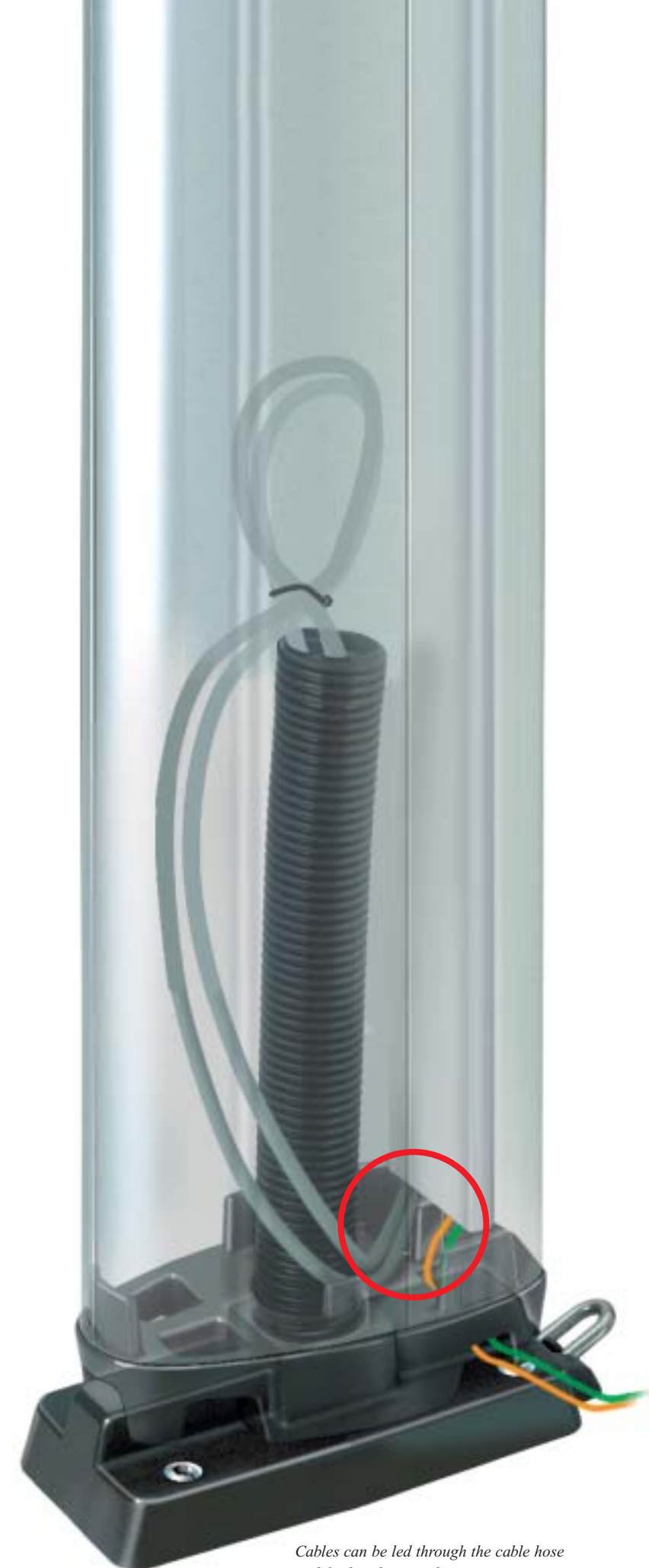
Small protrusion on top side of heel plug – acts as spacer for cable conduit. Allows cables to run freely.
